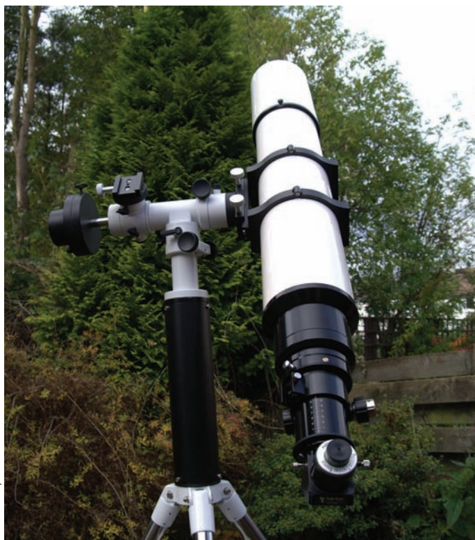
▲ APM's LZOS Model 152/1200D refractor on the author's alt-az mount. All images: Neil English.
