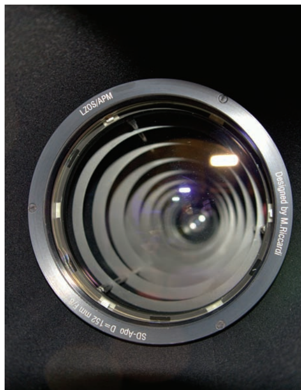
▼ A closer look at the telescope tube baffling.
