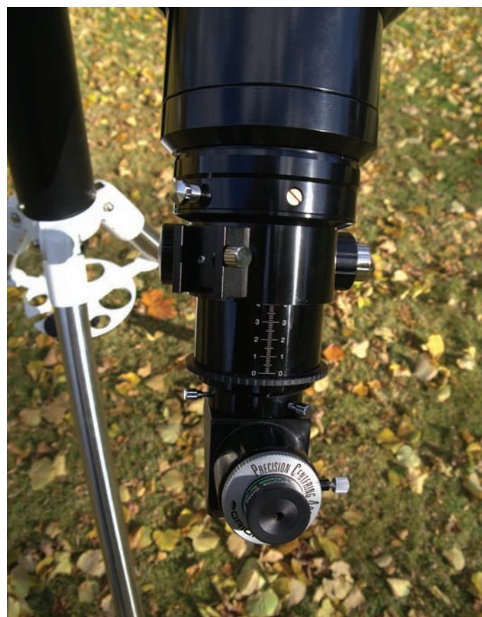
▲ The three-inch APM rack and pinion focuser.
