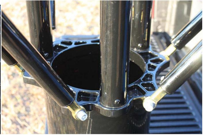
The 10 inch top is designed to accept most major brand mounts including Astrophysics among others. The entire top mount receiver plate rotates 360 degrees to assist in polar alignment. It is locked down with three plastic handled bolts.
