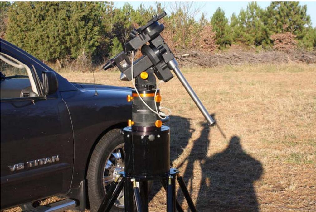
With two large scopes on a dual ADM mounting plate and 50lbs of counterweights ready to align and observe.
