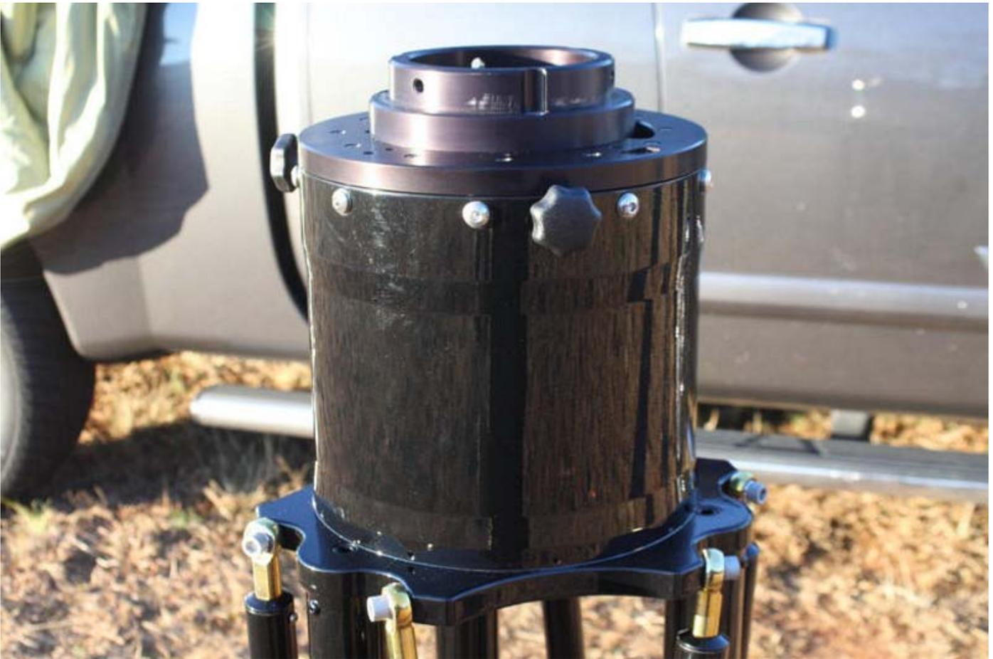
The legs have a very well designed individual leveling system which is a bolt with a locking nut on the top attached to a swiveling aluminum foot. It never budged a micron after the desired leveling height was reached.
